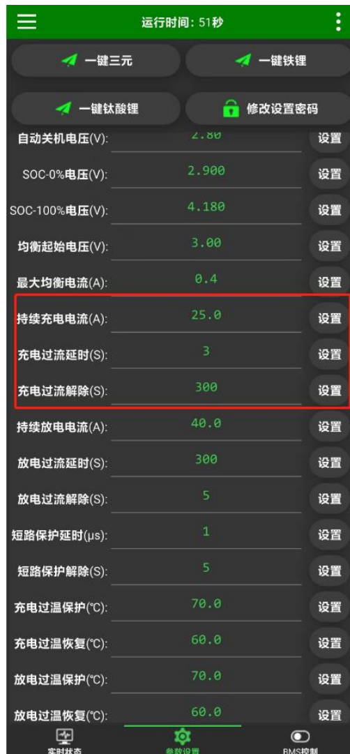
图6 APP设置保护板控制JK-BLMK-5A模块 Figure 6 APP Settings Protection board controls the JK-BLMK-5A module
